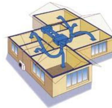
Ducted heat pumps (easier retrofit)
